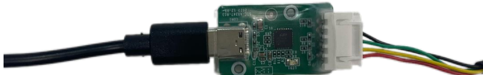
Figure 2-2 Connect the USB adapter to PC via USB Type-C cable
