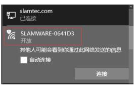
Please connect to the above SLAMWARE- XXXXXX network (you can also connect SLAMTEC MAPPER to PC via Ethernet cable. Please set the network mode as DHCP client).
